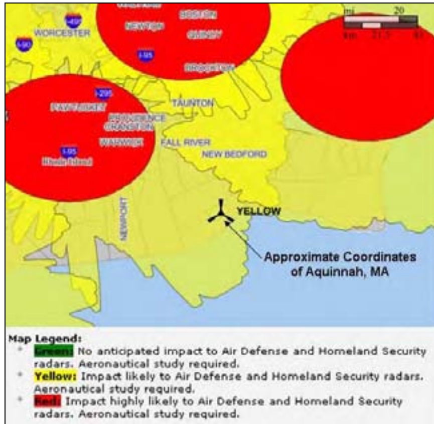
Figure 9. Preliminary Results of FAA Long-range Radar Impact Evaluation
