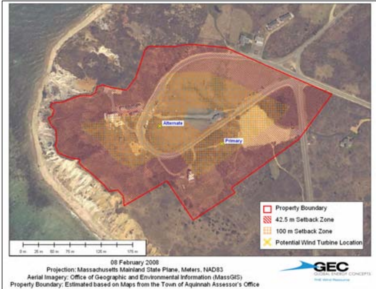
Figure 13. Setback Zones and Potential Wind Turbine Locations at Gay Head Cliffs
