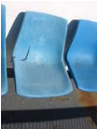
Sun damaged seat
