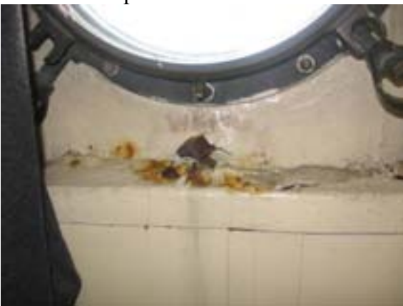
Hole in bulkhead under porthole
