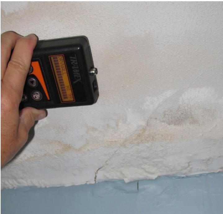
MM readings of 99% FS-DW in damaged ceiling area and wall below
