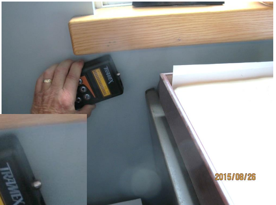
Elevated MM reading of 99% FS-DW under left corner of rear window in reception area indicating water seepage into cavity
