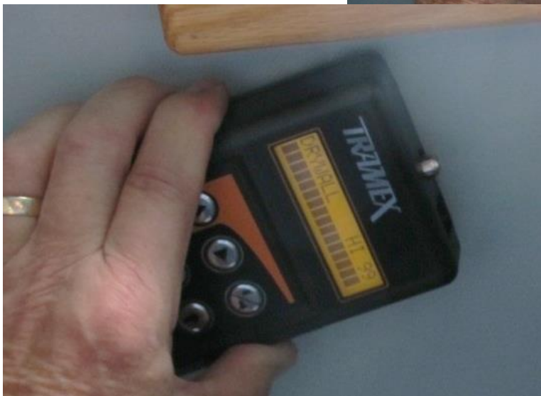
Elevated MM reading of 99% FS-DW under left corner of rear window in reception area indicating water seepage into cavity
