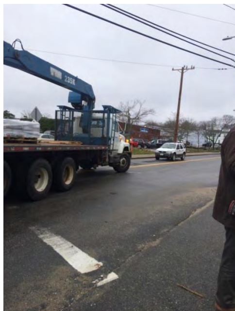
Large vehicle encroaching on eastbound Beach Street lane as it executes a right turn from Water Street onto Beach Street.
